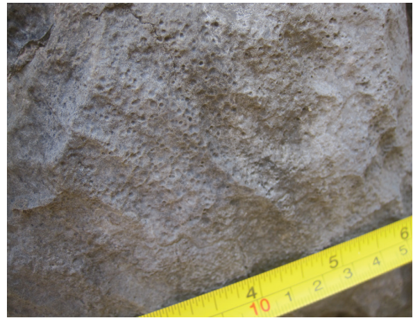
FIGURE 3. Frequent holes of millimetre diameter etched by lichens in the supratidal zone. Scale in inches and centimetres. Pulau Langgun
