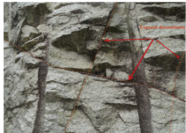
FIGURE 4. Exposed discontinuities of the granite slope. The behavior of the discontinuity joints influenced the ultimate bearing capacity of rock slope
