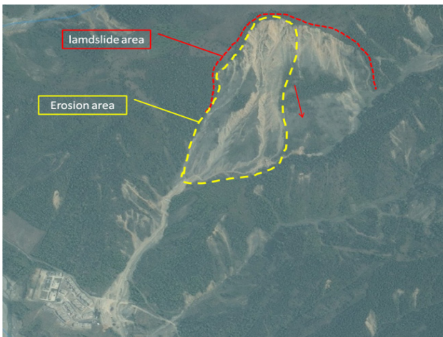
FIGURE 1. Fractured slope was eroded and led to retrogressive failures caused by rainfall and gravity along the gullies in the erosion area in Yindongzi Gully, Dujiangyan County, Chengdu City
