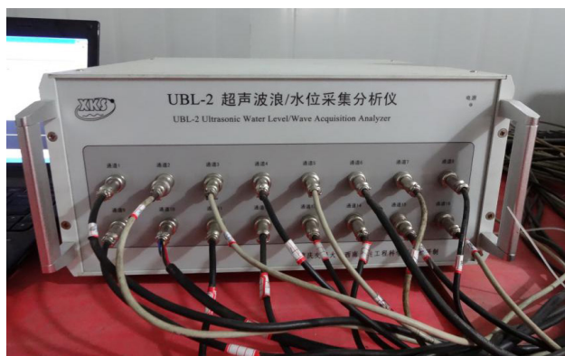
FIGURE 7. The ultrasonic wave collection and analysis device
