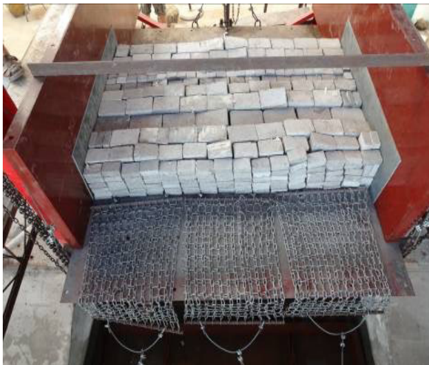
FIGURE 6. The landslide mass model
