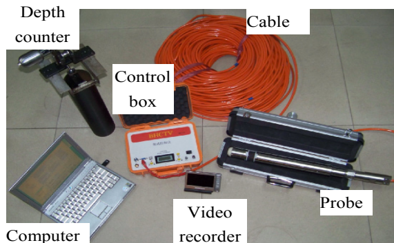
FIGURE 1. The digital panoramic borehole camera system
