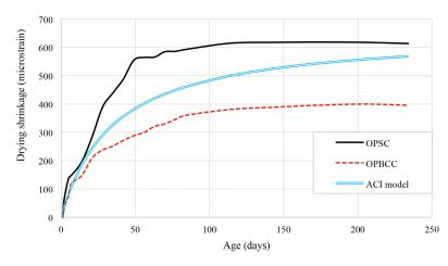
FIGURE 5. Drying shrinkage strain development of concretes
