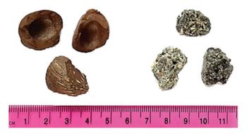
FIGURE 1. Oil palm shell (left) and oil-palm-boiler clinker (right)
