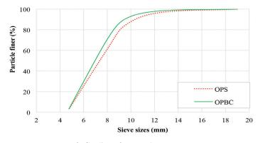
FIGURE 2. Grading of OPS and OPBC aggregates
