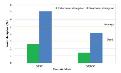
FIGURE 4. Water absorption of concrete mixes
