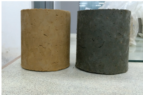
FIGURE 3. S3 Soil samples after compaction, the darker sample contains 0.2% CNF while the lighter sample has no NC
