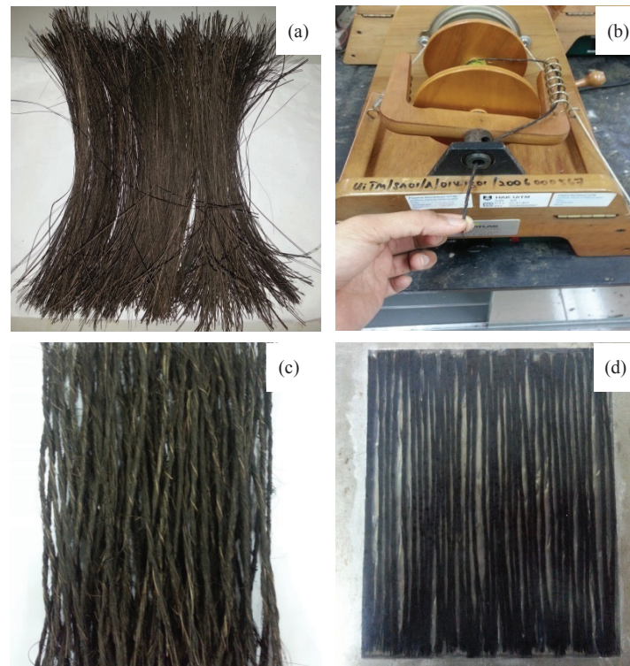
FIGURE 1. (a) A bundle of sugar palm fibre after combing, (b) yarning process, (c) sugar palm yarn fibre with 2500tex and (d) composite
