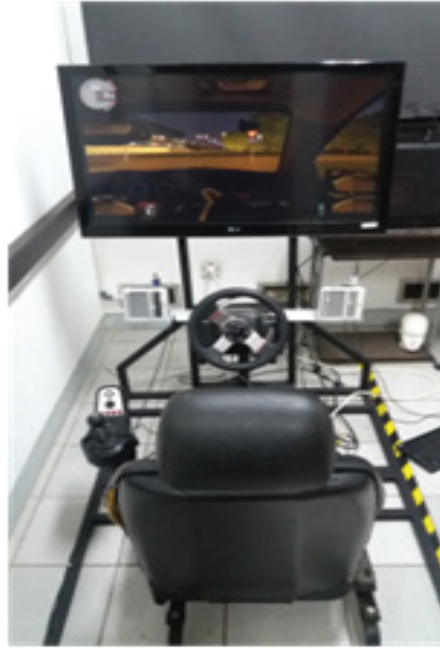
FIGURE 1. Simulator installation consists of driving simulator, LCD screen and a set blue lights on the dashboard
