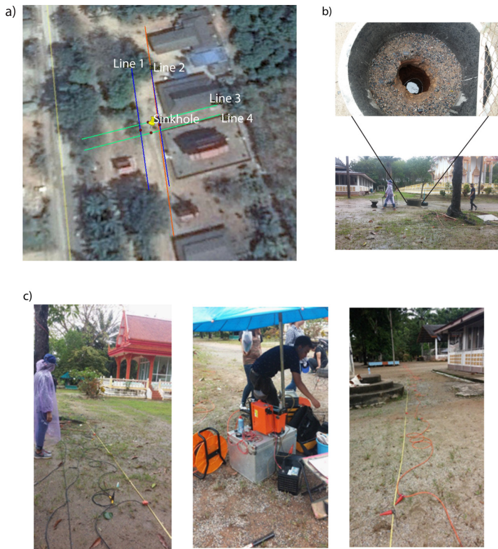
FIGURE 2. a) Geophysical survey lines, b) Sinkhole in the area, and c) Geophysical data acquisition
