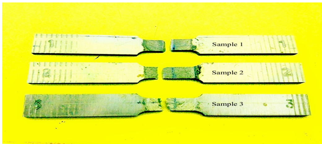
FIGURE 6. Fracture locations for samples 1, 2, and 3
