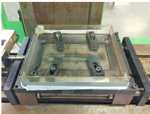
FIGURE 1. FSW fixture setup for experiments
