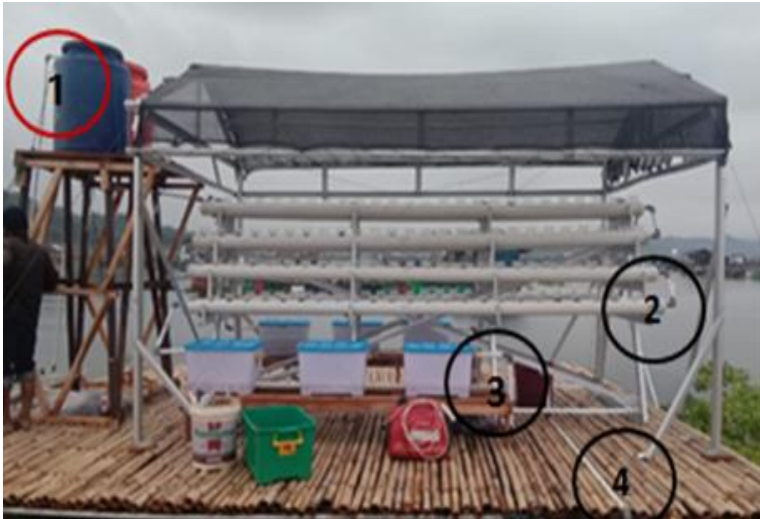
FIGURE 4. Point sampling of water quality was carried out once a week; (1) Water Tank as a reservoir of waste, (2) effluent of water spinach hydroponic, (3) effluent of the artificial wetland of vetiver grass, and (4) effluent of a physical filter
