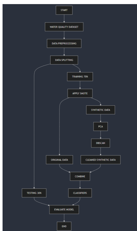
FIGURE 1. The flowchart of the proposed SMOTE-PCADBSCAN model in this study
